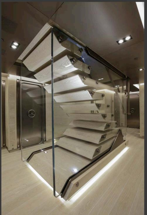
A dramatic feature on Sybaris are the staircases leading down to the lower deck and up to the fly bridge. Made of titanium with glass balustrades and treads of bleached American oak, the Class-approved laminated glass panels alone weigh over 600kg each, requiring reinforced beams fore and aft of the stairwell to support the structure.
